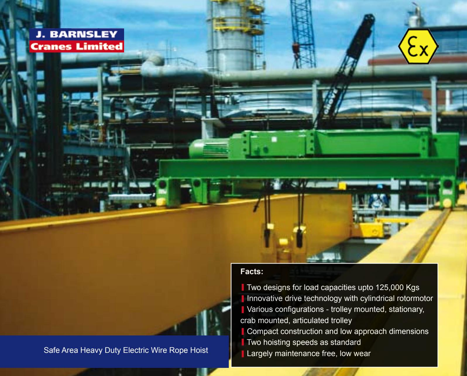
Safe Area Heavy Duty Electric Wire Rope Hoist
